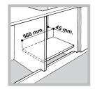
! The hob can only be installed above built-in ovens with a cooling ventilation system.
